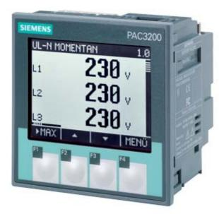
SENTRON, measuring device, 7KM PAC3200, LCD, L-L: 690 V, L-N: 400 V, 5 A, 3-phase, Modbus TCP, optional Modbus RTU / PROFINET / PROFIBUS, apparent/ active/reactive energy, class 0.5 acc. to IEC61557-12 or class 0.5s acc. to IEC62053-22, wide-range pwr sup. unit AC/DC, screw terminals
